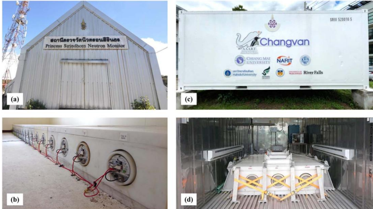
Figure 1. Photographs of the Princess Sirindhorn Neutron Monitor Station (PSNM) and the Changvan. (a) PSNM at the summit of Doi Inthanon, Thailand's highest mountain (2560 m above sea level). (b) Interior view of PSNM showing the 18-tube NM64. (c) Changvan at the Science and Technology Park, Mae Hia, Chiang Mai (340 m above sea level). (d) Semileaded (middle counter without lead producer) neutron monitor inside Changvan.
