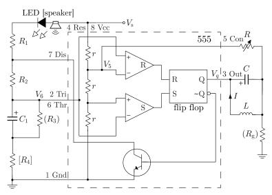
Diagram of the full circuit. In the (slightly simpler) minimal circuit, for which the LED flashes too quickly for the bifurcations to be studied by eye, components in parentheses are removed and those in square brackets are replaced by shorts.
