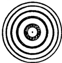
Figure 2: Interference Pattern Note: the actual interference pattern will most probably be more irregular and show less fringes.
